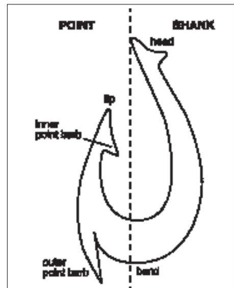
Figure 9. Parts of a one-piece fishhook.
